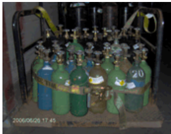
Figure 3B: The incorrect use of one strap around smaller cylinders
