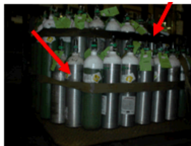
Figure 2B: The incorrect use of one strap around smaller cylinders.
