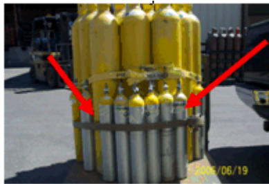
Figure 1B: Incorrect use of one strap around smaller cylinders.
