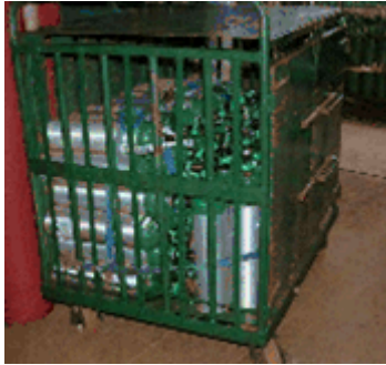
Figure 7: The correct way to secure cylinders on a cart .
