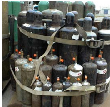
Figure 4B: The incorrect use of one strap around smaller cylinders.
