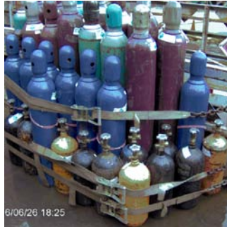
Figure 3A: The correct use of two straps to secure cylinders.
