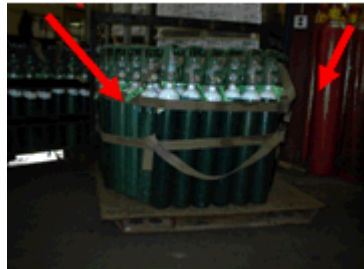
Figure 2A: The correct use of two straps to secure cylinders.
