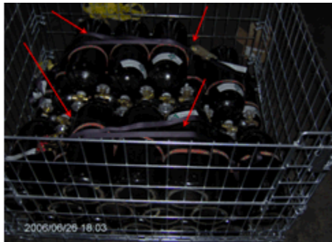
Figure 5A: The correct use of one 2" strap for each cluster of small cylinders, with the basket as a secondary securement device.
