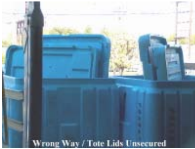
Figure 8-5: Unsecured Dry Ice Bin Lids
