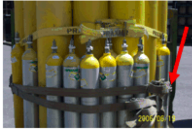
Figure 1A: The correct use of three straps to strap and secure a load.
