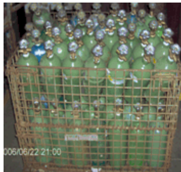
Figure 5B: The incorrect placement of cylinders in a basket without securing them with a primary strap. Never stack cylinders on the valves of other cylinders.
