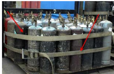
Figure 4A: The correct use of two straps to secure cylinders.
